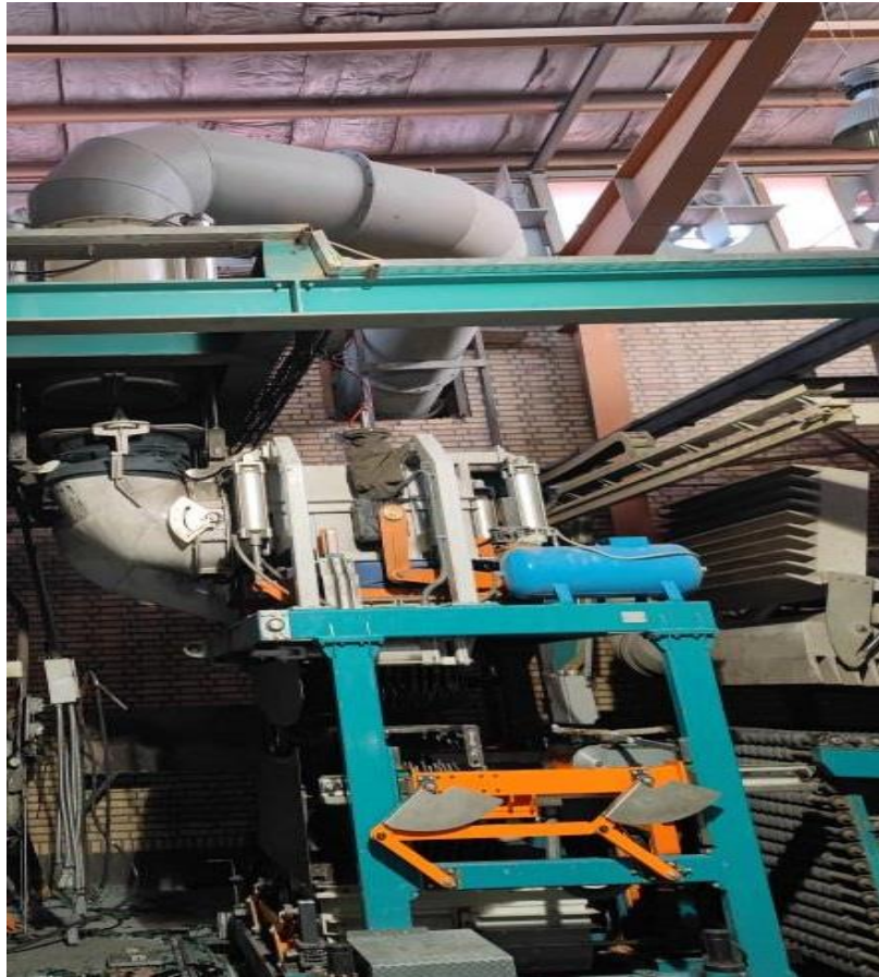
Fig. 2. Last section of a furnace for automotive glasses (front side) where the blowers inject the compressed air over the hot glass (courtesy of Venus Glass Co.)
