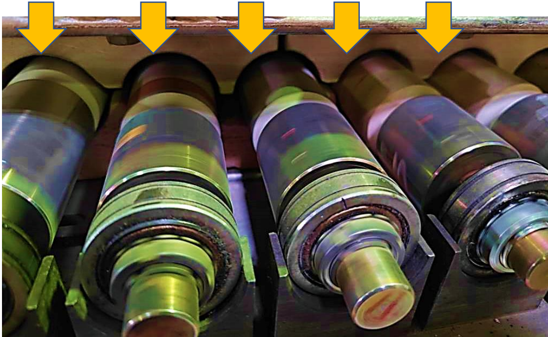
Fig. 4. A close-up image emphasizing on the ceramic conveyor rolls coupled with metal pliers in both ends of the ceramic (original image depicted at 200% color saturation and 50% sharpening correction)
