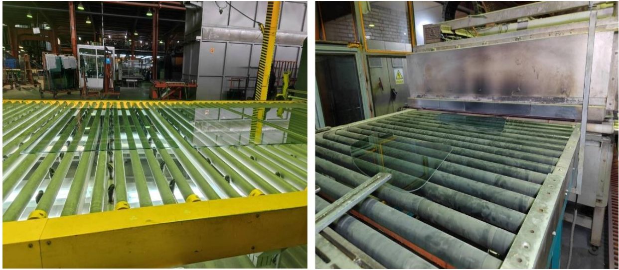
Fig. 1. Architectural and automotive glass production lines (glass loading section – entry of the furnace) at Venus Glass factory, respectively
