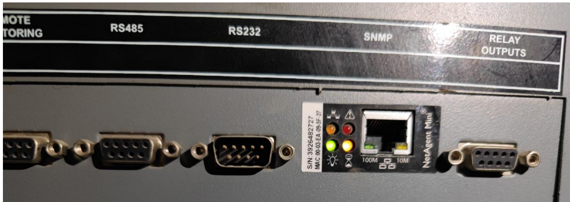
Fig. 6. Backplate of a UPS containing different sockets or communication endpoints for different communication protocols
